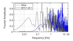
Figure 5: Normalized Fourier Amplitude spectra of two considered windward and simulated earthquake records.
